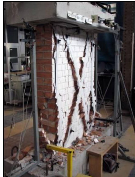
Figure 16. Delamination of CFRP strips at ultimate state
